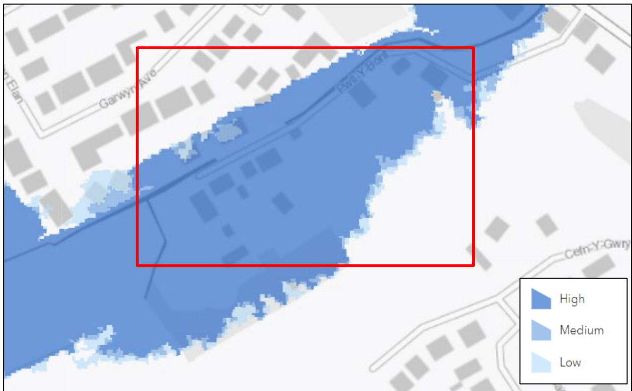
Figure 40: NRW Flood Risk from Rivers at the Pwll y Bont Investigation area
