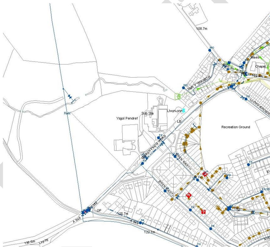
Figure 7: Local water and sewerage network
