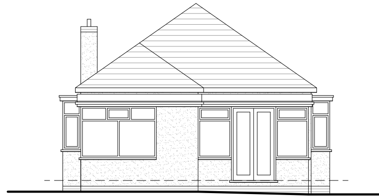
EXISTING REAR ELEVATION
